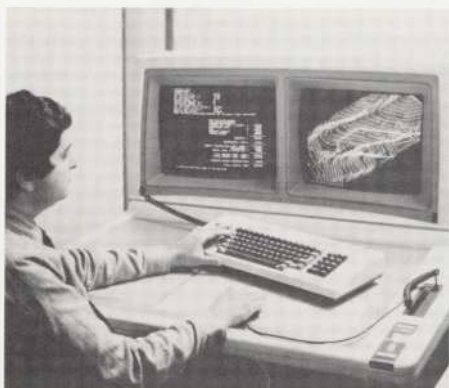
Double-screen allows engineers to see data and topography simultaneously.
