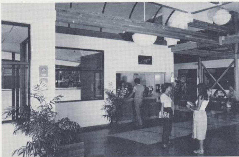
Interior view of the main waiting area showing exposed glu-lam beams and steel bracing frame lighted by curved glass skylights.
