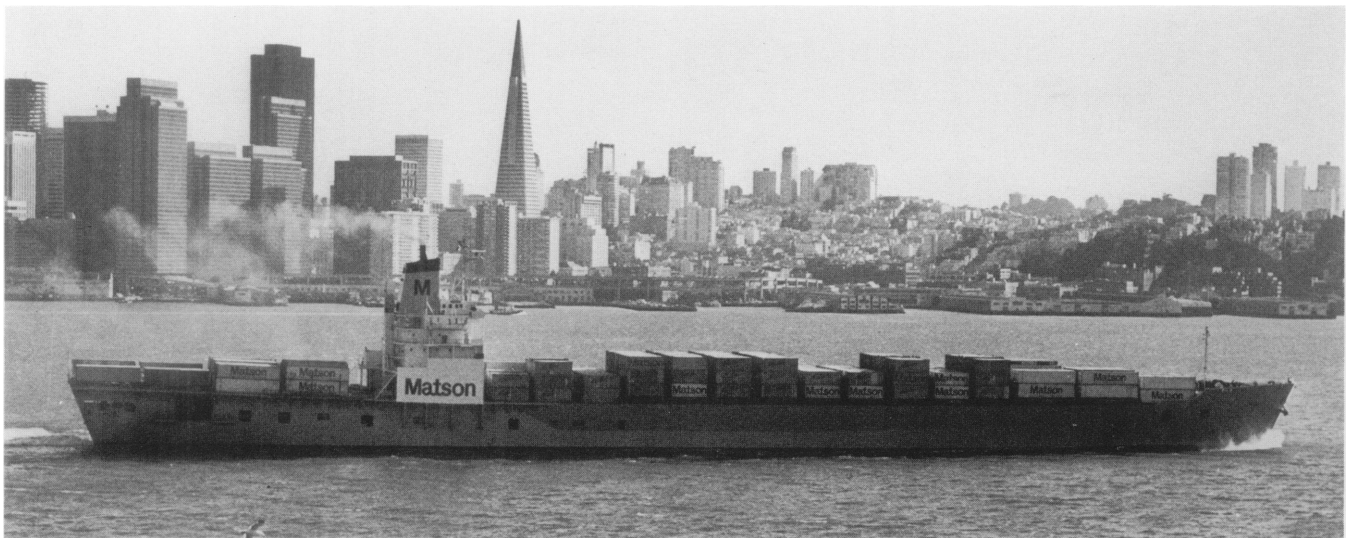
Today's LURLINE, fifth Matson vessel to bear the famous name, is a combination roll-on, roll-off trailership and container carrier. Vessel was converted from a "ro-ro" and "stretched out" with 126½-foot midbody in 1981 to add lift-on, lift-off capability and triple cargo capacity.
