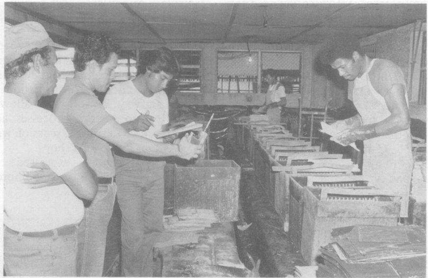
Nicaraguan Ministry of Labor inspectors monitor the air for sulfuric acid mist at the Willard lead battery plant, using a donated Draeger pump. (Photo: Karen Cohn.)
