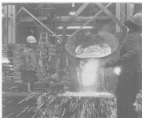
Molten metal is poured directly from ladle suspended from overhead crane into molds.
