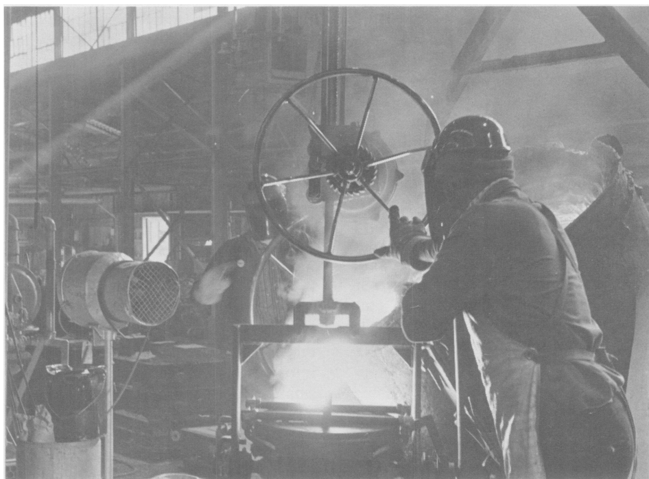
Tapping of ladle may cause burns or expose workers to fumes, noise and ultraviolet radiation.
