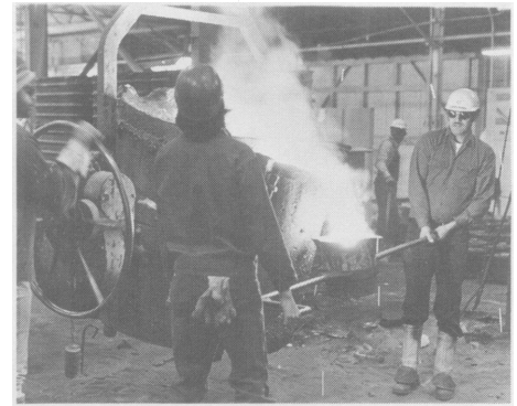
Metal being transferred to hand-operated ladle for small intricate castings. Heavy metal poisoning takes its toll among foundry workers.
