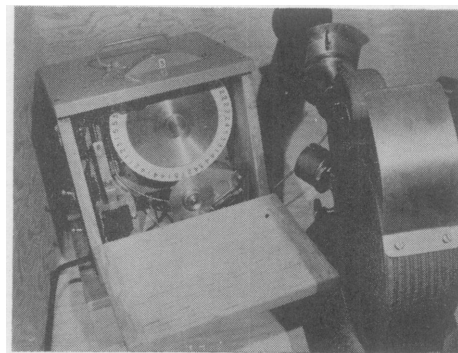
FIGURE 3. DETAILED VIEW OF THE MECHANISM OF THE STIMULUS TIMER
