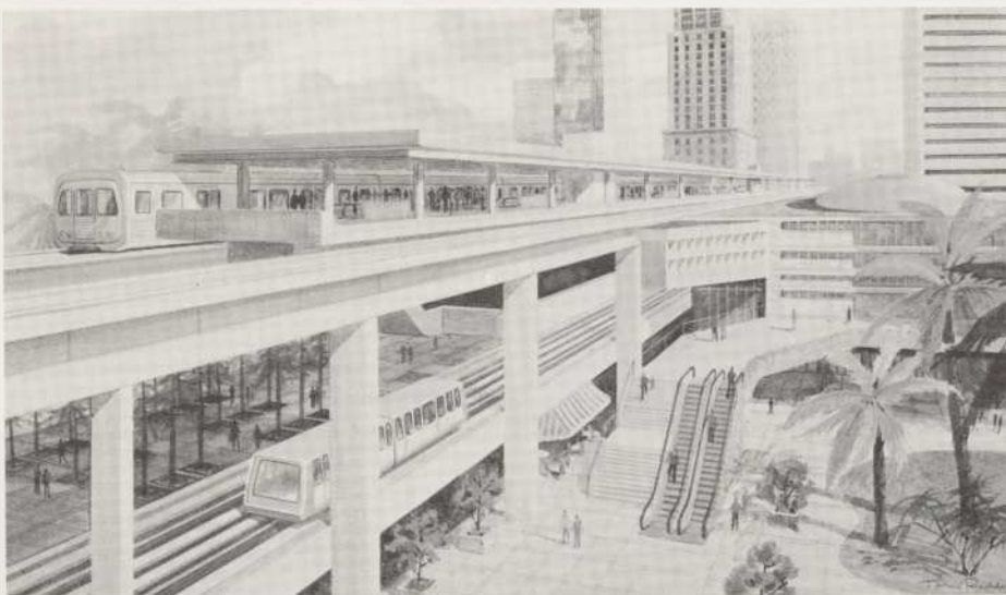
The Miami Metrorail (upper level) and Downtown People Mover (lower rail) will interface at Government Center Station, as shown in this artist's rendering.
