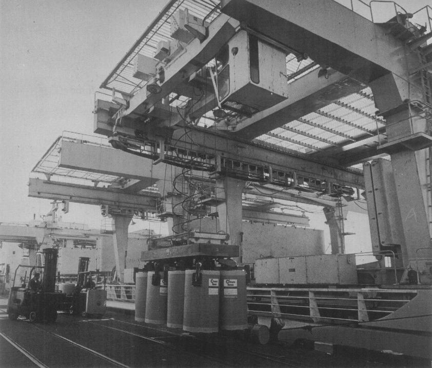
Three gantry cranes aboard the SS Bessegen can work at the same time. Totally automated hydraulic hatch covers open the ship for work in the matter of moments and each crane can load or discharge 200 to 250 rolls of newsprint per hour as against 60 to 70 rolls by the conventional method.
